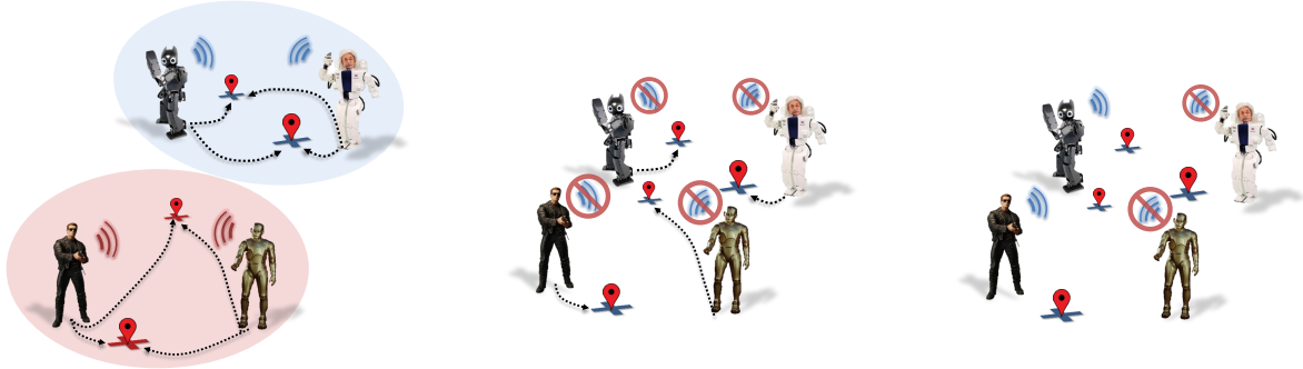
(a) Finding partitions a team to bound communication within the sub-teams (red and blue ovals) (b) Understanding the cost incurred by forgoing further communication and sticking with the initial assignment (arrows) (c) Limiting communication to nearby robots to determine if the current assignment is still optimal despite cost changes
