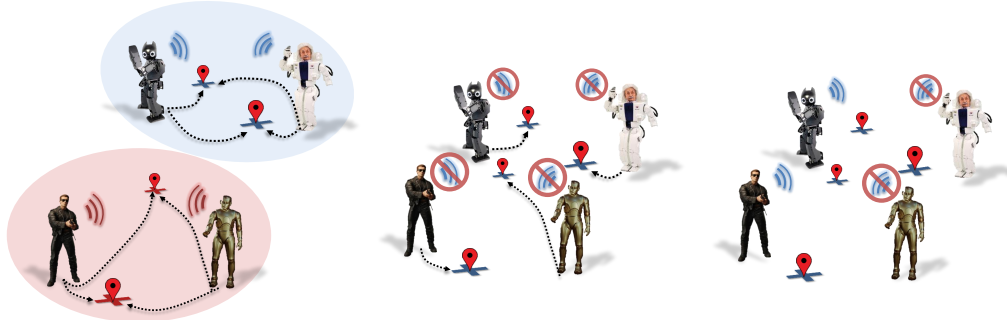
(a) Factorizing a team into smaller cliques. (b) Persisting an initial assignment. (c) Local communication to check optimality violations of costs.
