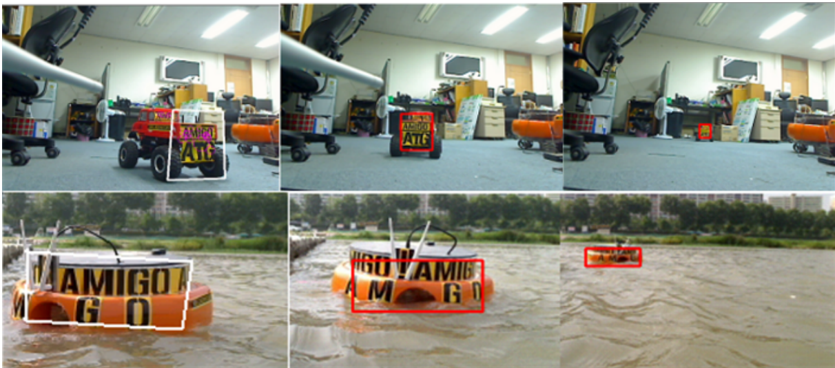
Figure 10: Target detection (white boxes) and tracking (red boxes) for the AGV and ASVs. Left: Target Detection at 1m. Middle: Target Tracking at 2m. Right: Target Tracking at 4m.
