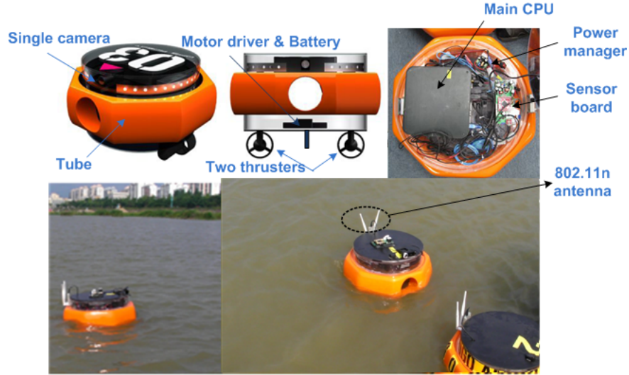
Figure 3: Autonomous Surface Vehicle designed as a prototype system in order to assess the feasibility of a robotic containment boom deployment. These units are the primary platform used for implementation, development and validation of the robust visual servoing and docking behaviors.
