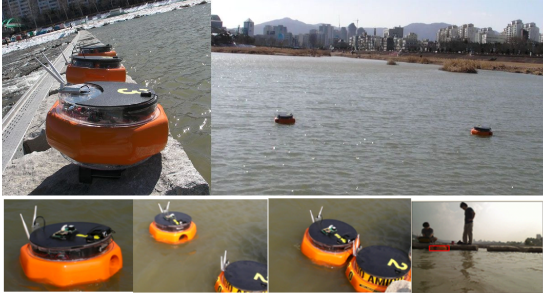
Figure 14: An example USV pair docking test. (Compare the water surface to the calm day shown in Figure 4.)
