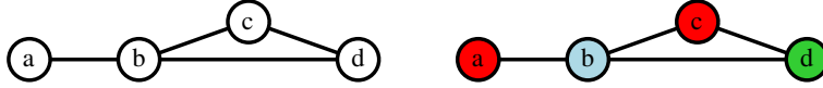
Figure 14: [left] An example instance of the 3-coloring problem. [right] A coloring of that graph using three colors.
