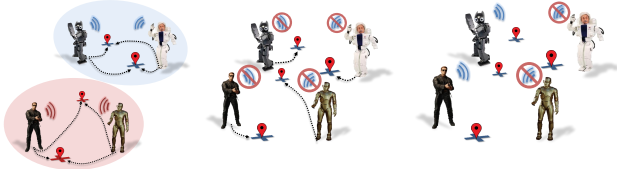
(a) Factorizing a team into smaller cliques. (b) Persisting with an initial assignment. (c) Determining optimal-ity violations locally. Fig. 2: Three methods to reduce MRTA centralization. (a) Cliques are sought by analyzing \theta(X_q^*) with a given C . (b) The worst case maximum sub-optimality is computed should robots persist with their assignment. (c) Robots use local communication to check whether the changed costs now violate the current \theta(X^*) .
