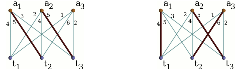
Fig. 2: (left) Two matched edges found after running two stages of the algorithm; (right) A perfect matching consisting of three matched edges is found after one more stage (by augmenting path a_3 \rightarrow t_2 \rightarrow a_1 \rightarrow t_1 ).
